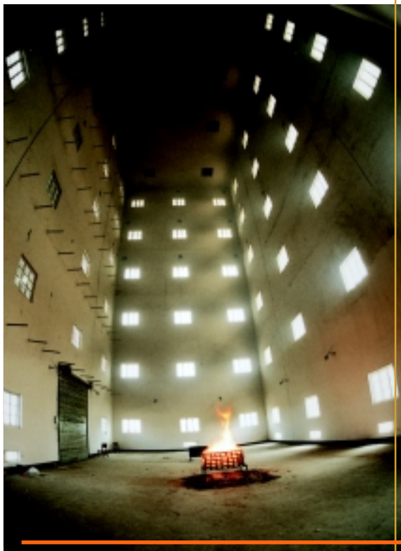
An experiment of natural smoke filling process. 自然灌煙實驗
