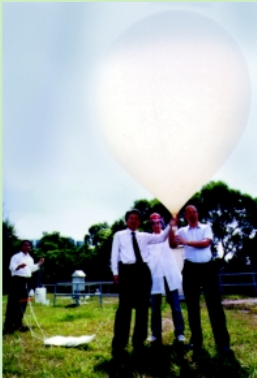
One of the research projects being undertaken at the Centre. The balloon is ready to be released for ozone analysis.
