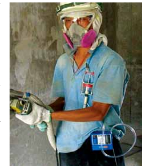
Sampling during grinding process 在研磨工序中收集吸入人體的塵埃樣本
