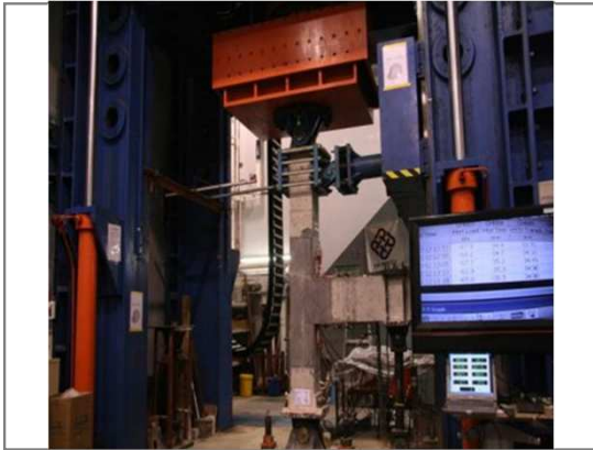
10000kN Servo Control Multi-purpose Testing System (MPTS)
