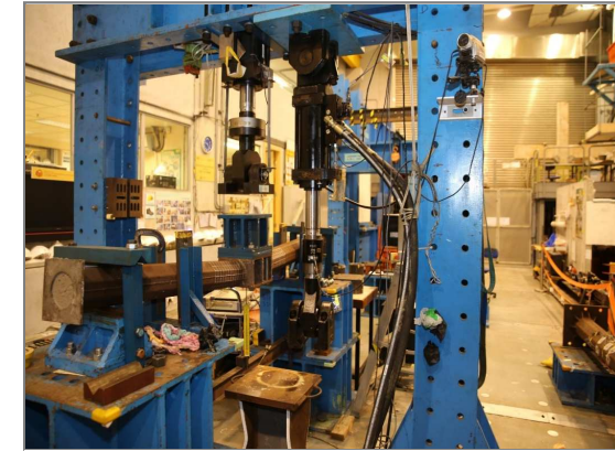
100 ton loading frame
